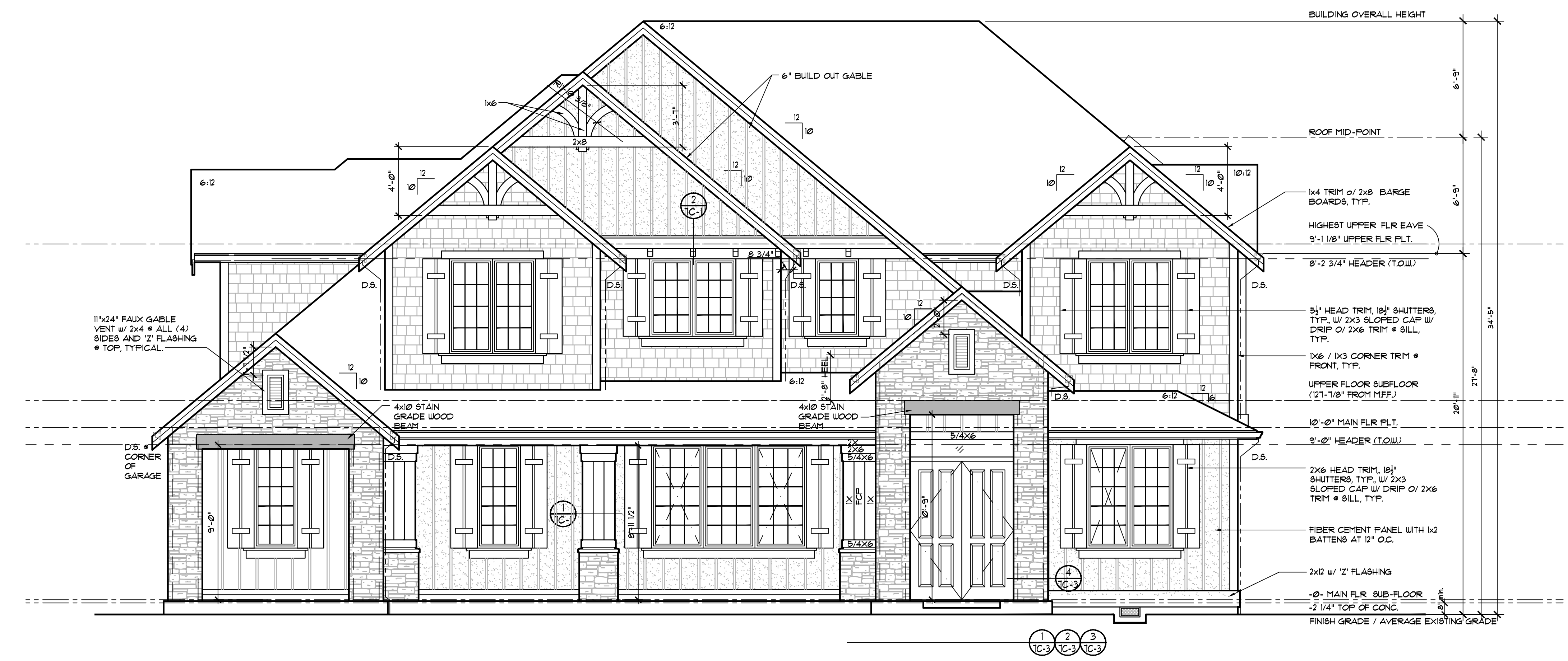
FRONT ELEVATION 'C-04RSG' 1/4" = 1'-0"
